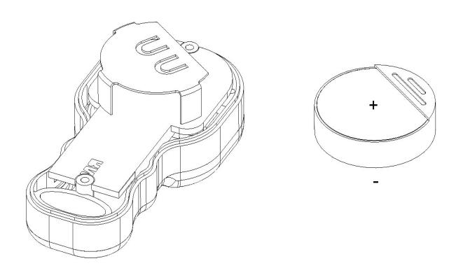
7. Install the new batteries. Push the batteries into the circuit board (make sure not to use to much force)
