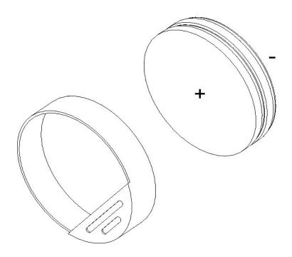
6. When installing the new batteries, make sure they are in the proper configuration. Positive facing up, and negative facing down.
