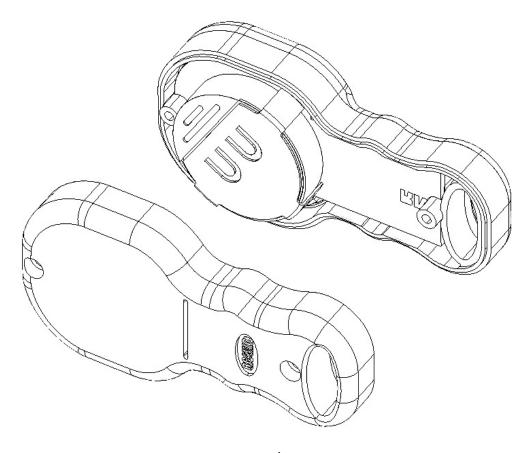
3. Wiggle the circuit board back and forth making sure to keep it flat/horizontal with the case front. This process is very important to raise the electronic board just enough to remove the battery. You do not need to fully remove the circuit board.
