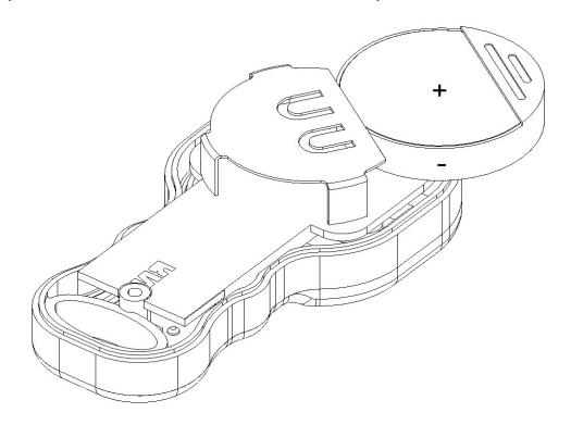
Note: The positive needs to be facing up, and the negative side facing down on both batteries.
