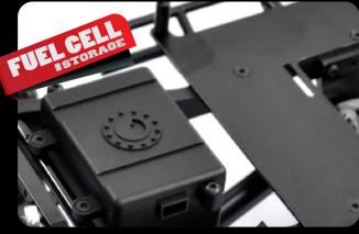
The TF2 Chassis features a molded fuel cell that doubles as an electronics storage box plus an aluminum, frame-mounted under cab electronics tray for multiple electronics mounting options.
