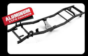
The All New TF2 Chassis is a machined billet aluminum ladder frame design with leaf springs, scale shock hoops, chassis servo mounts and hard body mounts. 4-link conversion available soon!
